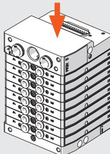
Position the valves in the desired sequence, making sure the small teeth "A" of each guard engage with the next one and in the seat of the blind terminal. Also check that gasket "B" rests in its seat. Place the blind terminal on a flat surface. Apply a thrust of several kilograms on the input terminal to compact the valves properly one against the other.
